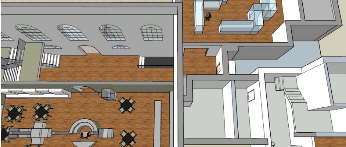
Figure 33: A new entrance hall and lift lobby giving access to the Basement and First Floor Level
